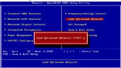
**NOTE:** Load Optimized Defaults loads the default system values directly from ROM. If the stored record created by the Setup program should ever become corrupted (and therefore unusable). These defaults will load automatically when you turn the PCA-6780 system on.
